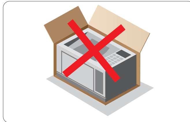
Product with no inner filling: the risk of damage is very high!
